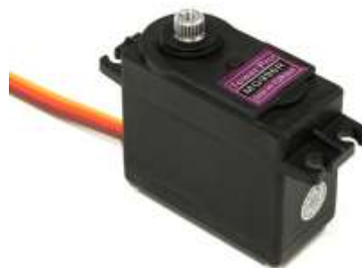
Gambar 2. 3 Motor Servo MG 996 R (Sumber : Servo Data Base, 2018)
